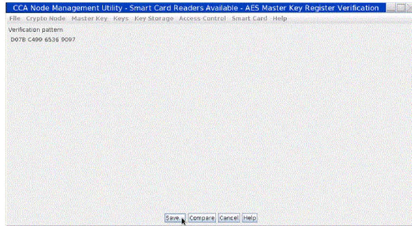
Figure 212. Master Key Register Verification panel - verification pattern is displayed
