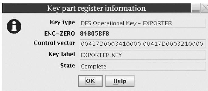
Figure 127. DES Key part register information - predefined EXPORTER key type in Complete state
