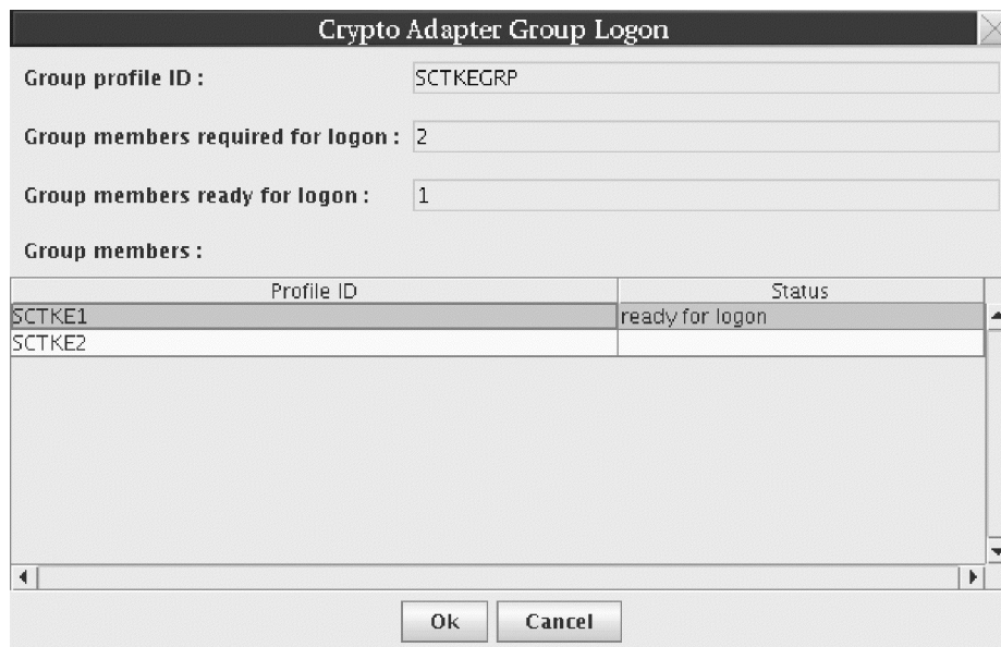
Figure 41. Crypto Adapter Group logon window with smart card profile ready
